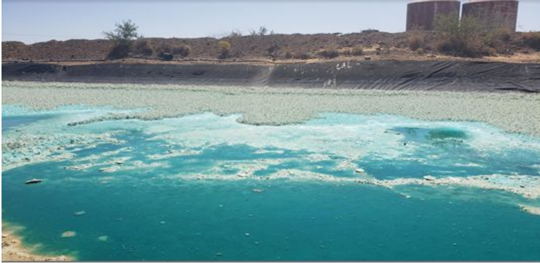
Figure 3.6: Pregnant Leachate Pond (photo credit - Sydney Adamonis)
